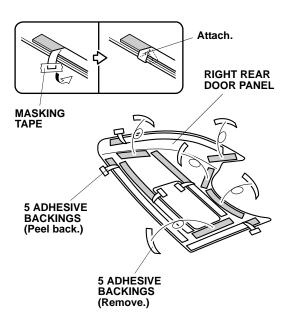
30. Align the right rear door panel and attach it as shown.
