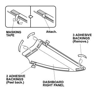
11. Align the dashboard right panel and attach it as shown.
